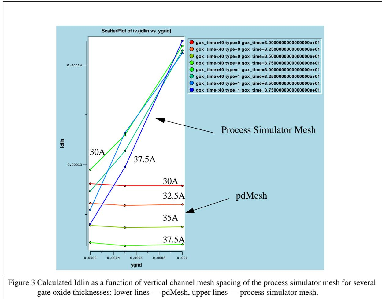
Oscillations of the Idlin versus Tox curves calculated using the process simulator mesh clearly show the effect of the oxide interface traversing successive mesh lines. Each time this happens, a spike is observed in the curve.
