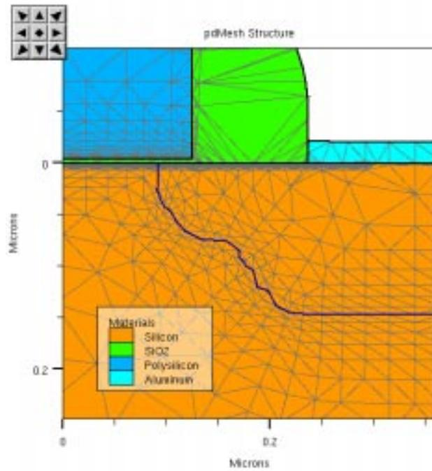
Figure 2 pdMesh generated MOSFET mesh
