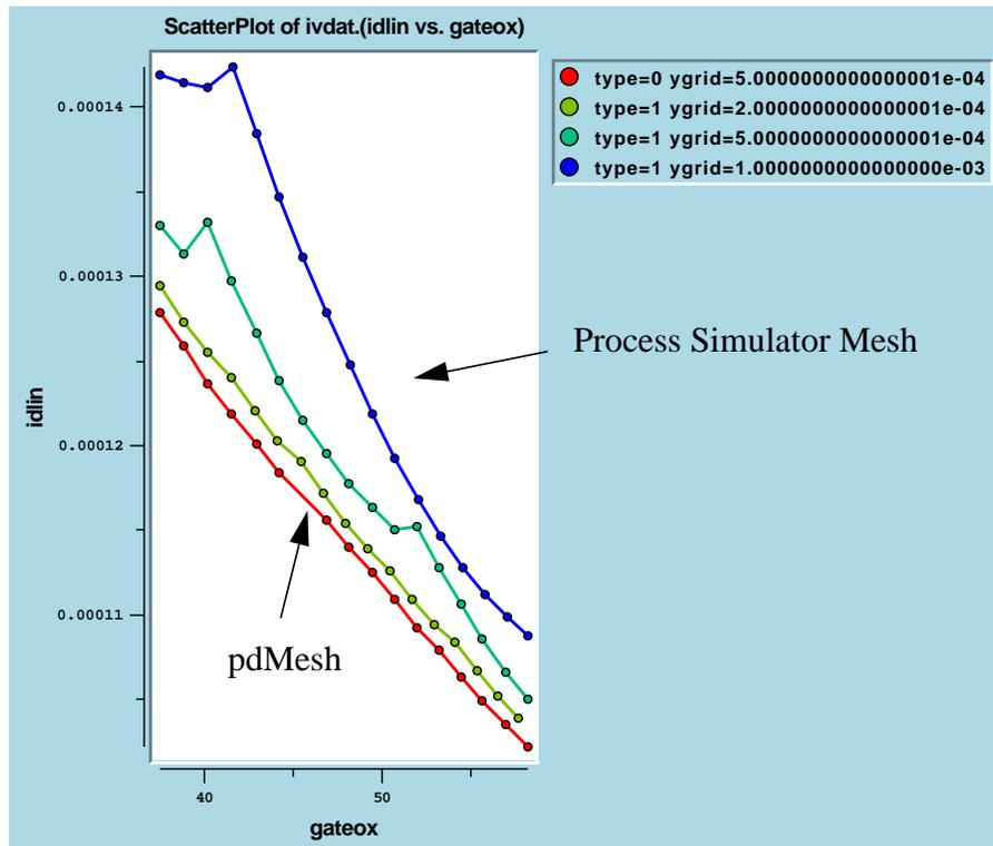
Figure 4 Calculated Idlin as a function of gate oxide thickness: lowest line — pdMesh, other lines — process simulator meshes with 2A, 5A and 10A vertical mesh spacing in the channel.
