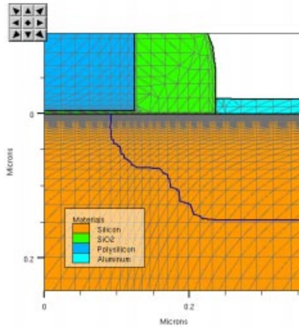
Figure 1 Process simulator mesh near the gate corner.
