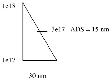
**FIGURE 1.** Assume the dopant concentration varies by 1 decade every 30 nm. For a background concentration of  $3e17$  atoms/cm<sup>3</sup>, the average dopant spacing (ADS) is 15 nm. Thus, near the junction, the dopant concentration is changing by 3x over the ADS.
